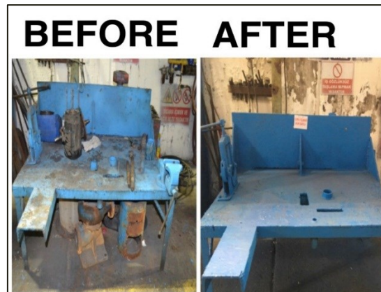
Figure 5.: Implementing of 5s in the material area(Shine)
