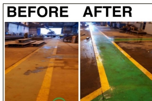
Figure 6.: Implementing of 5s in the pathway(Safety)
