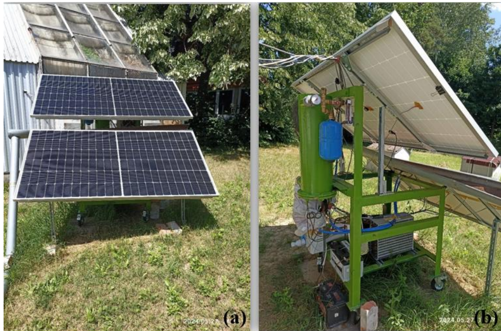
Figure 1. Experimental Setup, a: PV and PVT, b: back side of both panels
