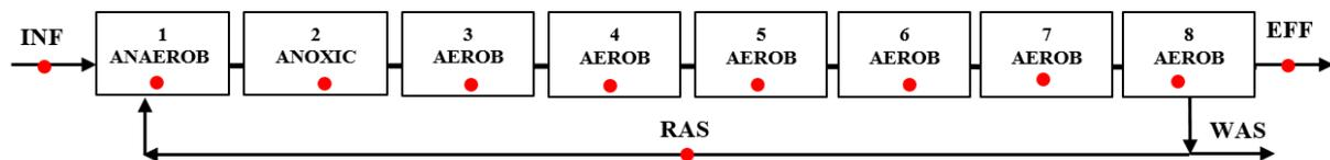
**Figure 3. Process scheme of the sampled part of the continuous activated sludge wastewater treatment plant with sampling points (red dots)**
