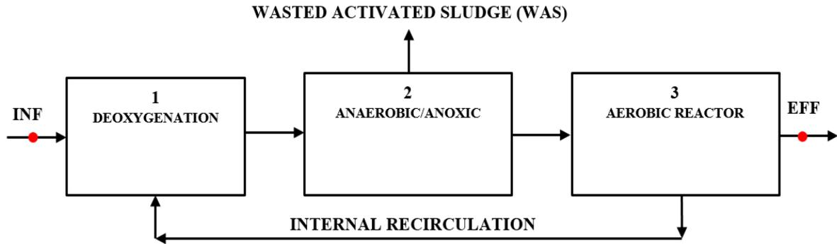
**Figure 1. Process scheme of Organica Fed Batch Reactor, semi-continuous system with sampling points (red dots)**
