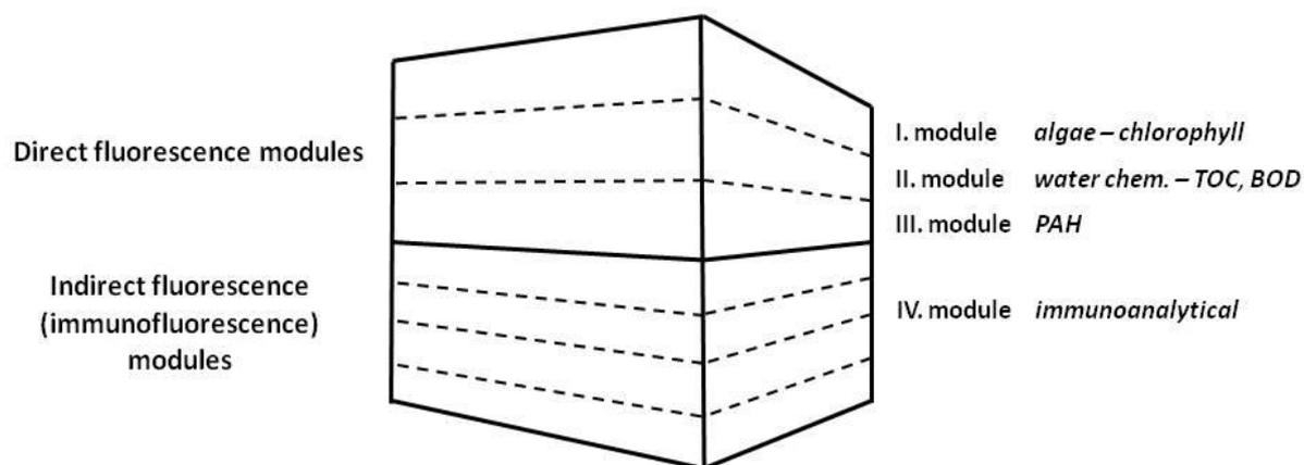
**Figure 2. Schematic setup of the modules of the fluorometer prototypes.**
