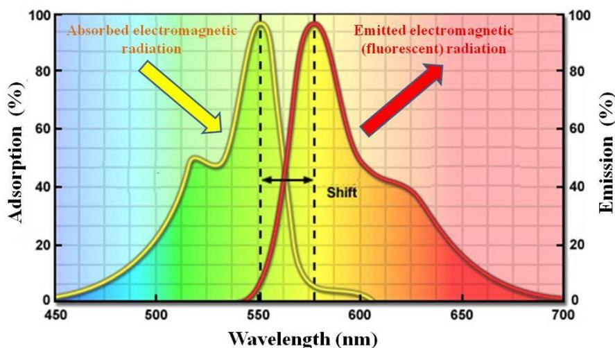
**Figure 1. Fluorophore absorption and emission profiles.**
