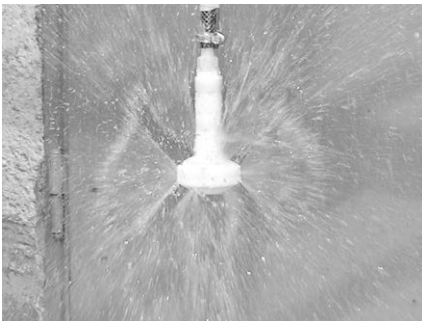
Photo 7 ARAG nozzle during operation
