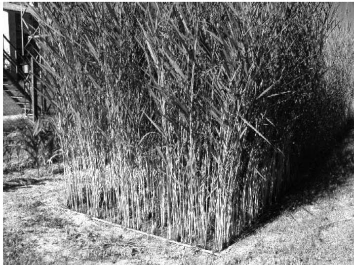
*Fig. 1 The tank (growing chamber) of the evapotranspirometer with the reed stand*
