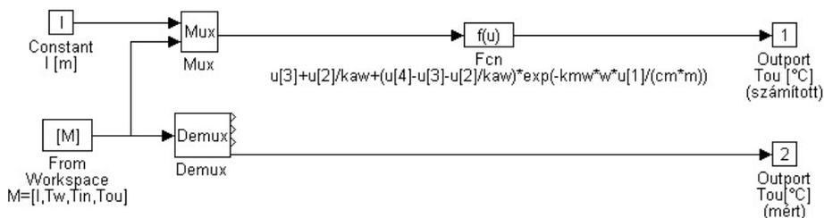
Figure 3: The model of the solar collector in Simulink
