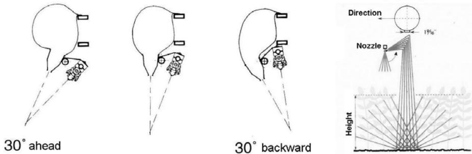
*Fig. 11 Air-assisted spraying*
