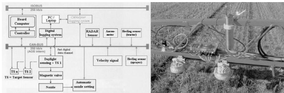
*Fig. 7 Schematic overview of the electronic net of the multi-sensor system and individual plant sensors.*
