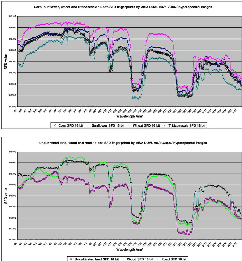
Figure 4. Spectral 16-bit SFD 'fingerprints' of corn, sunflower, wheat, and tricosecale (above picture) and of uncultivated land, wood and road (bottom picture) based on AISA Dual data
