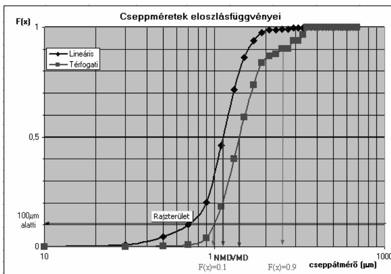
Fig. 14 Droplet structure by a rotation nozzle of type Micron X1 at rpm  $n=1410$  l/min.
