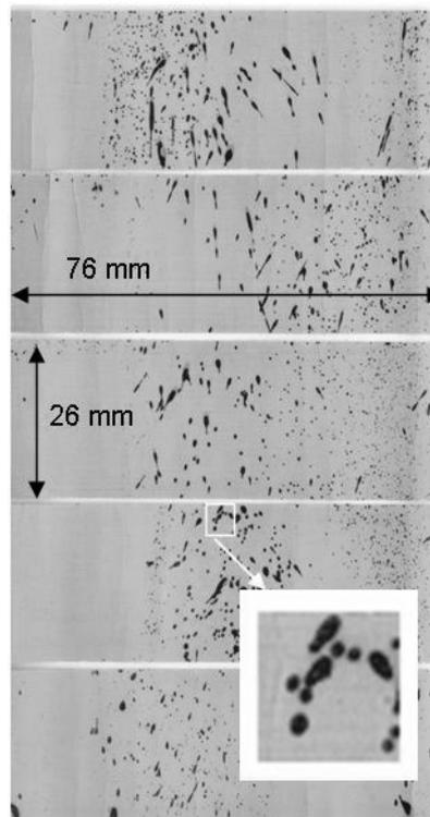
*Fig. 12 Water sensitive paper sample used at investigation of a TX ConeJet VK 26 type nozzle at work.*
