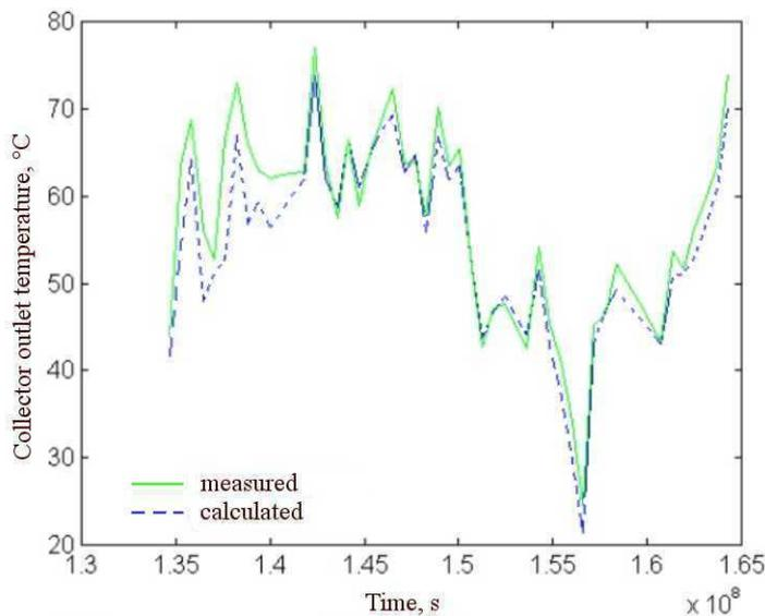
Figure 4: Collector outlet temperature before parameter identification, when  $k_{aw}=k_{mw}=1$
