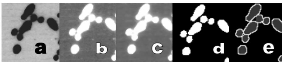
Fig. 13 (a) color to gray transformation, (b) inverse picture (easier to follow visually), (c) noise reduction, (d) detection and watershed, (e) transformation.
