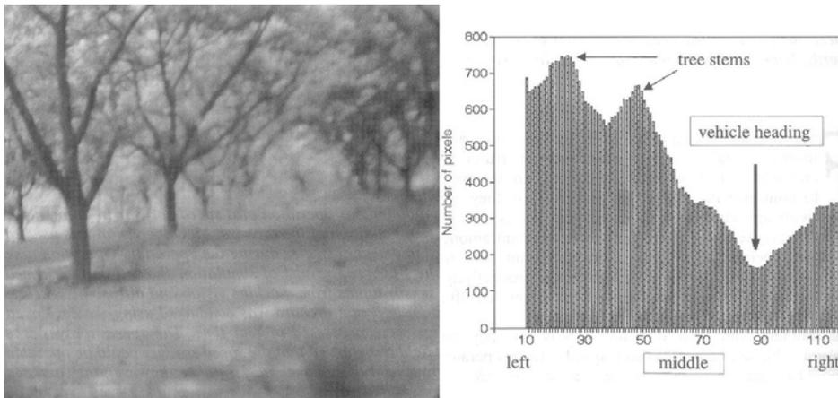
*Fig. 9 Machine vision and image processing to determine moving direction of an autonomous sprayer.*
