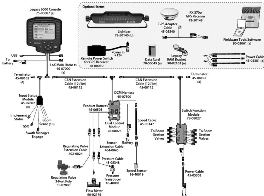
Fig. 3 Schematic overview of FieldPilot on a plant protection sprayer.
