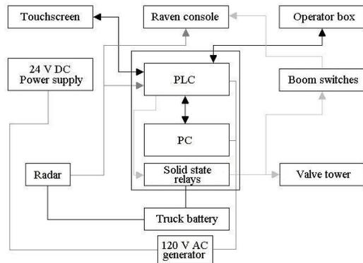
*Fig. 8 Schematic overview of the real-time control.*
