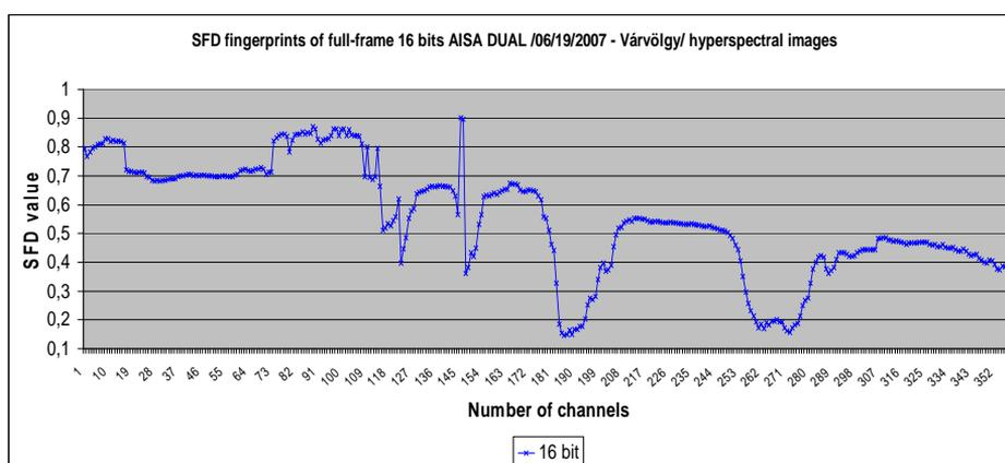
*Figure 5. 16-bit spectral SFD fingerprint of the whole AISA Dual image (19. June 2007, Várköly) for the identification of noisy bands*
