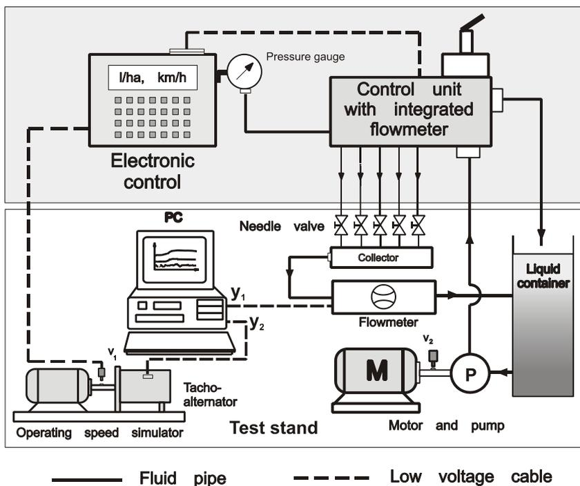
Fig. 1 The dosage regulating and measuring apparatus
