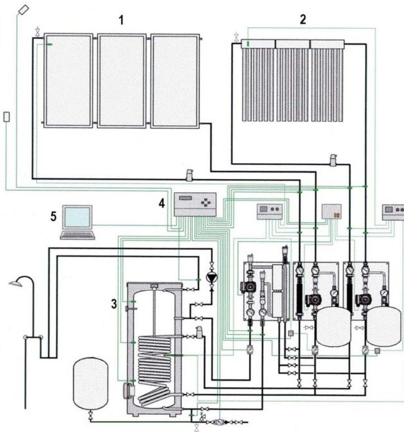
1. flat plate collectors; 2. vacuum tube collectors; 3. hot water tank;
