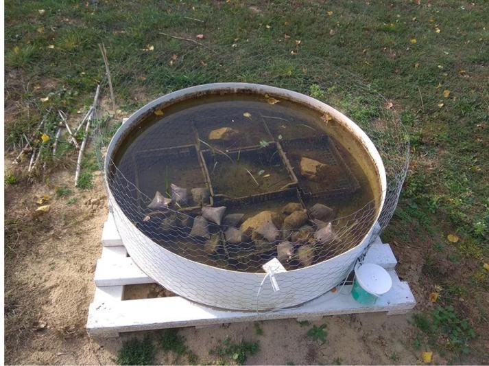
*Figure 1.: Class „A” evaporation pan with litterbags*
