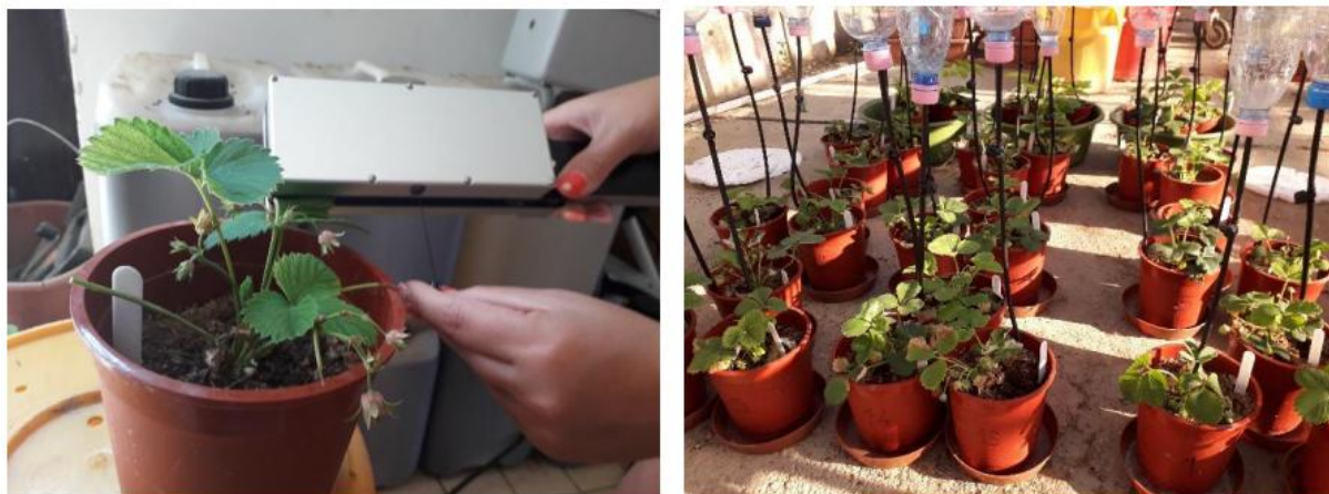
Figure 1 Leaf area measurement using an LI-3000C device and the installed drip irrigation system.
