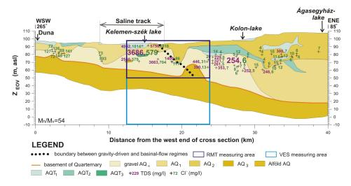
Fig. 4. TDS and Cl<sup>-</sup> content of the groundwater
