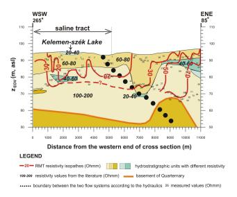
Fig 6. RMT measurements
