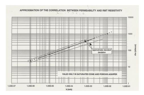
Fig. 2: Approximation of hydraulic conductivity obtained with RMT resistivities. Correlation is valid only with electrical conductivity of the water between 500-800 μS/cm at 25 °C.
