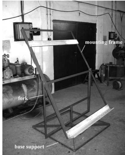
Figure 2. Mounting frame of the simulator (University of Pannonia, Georgikon Faculty, Department of Agricultural Mechanization)
