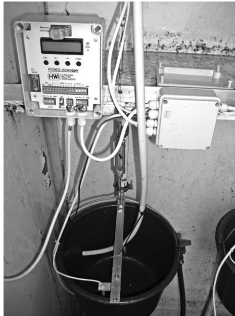
Photo 1. One unit of water supplier with the data logger of the evapotranspirometer (Photo: G. Soós)
