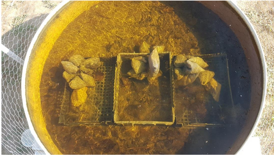
Figure 3: Class A evaporation pan with the litter bags fixed to plastic racks
