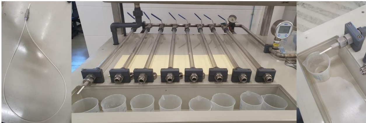
Fig. 4. Membrane sample prepared for measurement, permeability measuring device and measuring cup for permeate water
