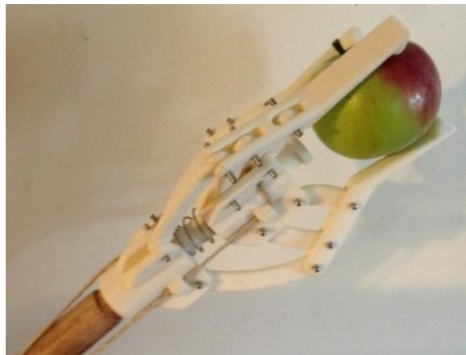
Figure 2. Fruit picker from 3D printed material and wood.
