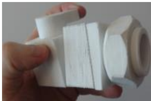
Figure 3. A 3D printed spigot.
