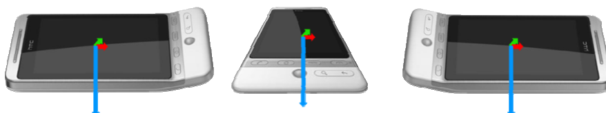
Figure 2: Equivalent orientations for the g-sensor
