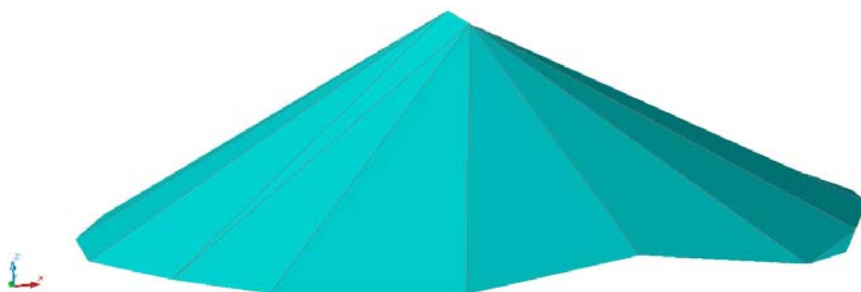
Figure 8: AutoCAD Civil 3D programme, the superficies fitted to a set of points of a regular depot
