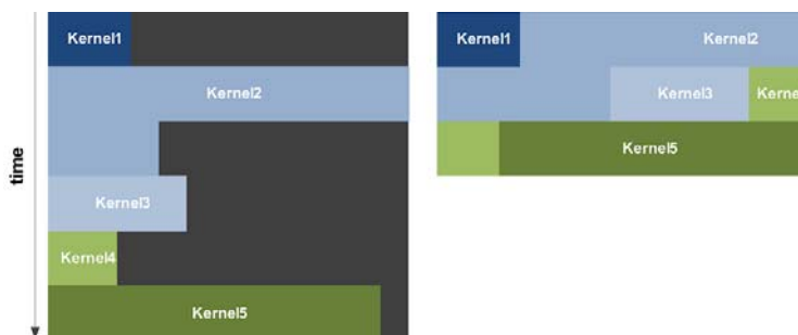
Figure 4: Parallel and concurrent execution of the kernel.
