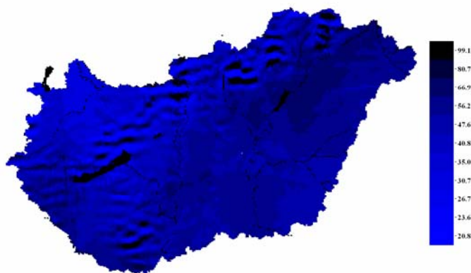
Figure 7: Average production costs (in HUF) of 1 kWh electrical energy considering all the expenditures arisen and all the electrical energy produced during the lifetime of the wind power plant described in the text.
