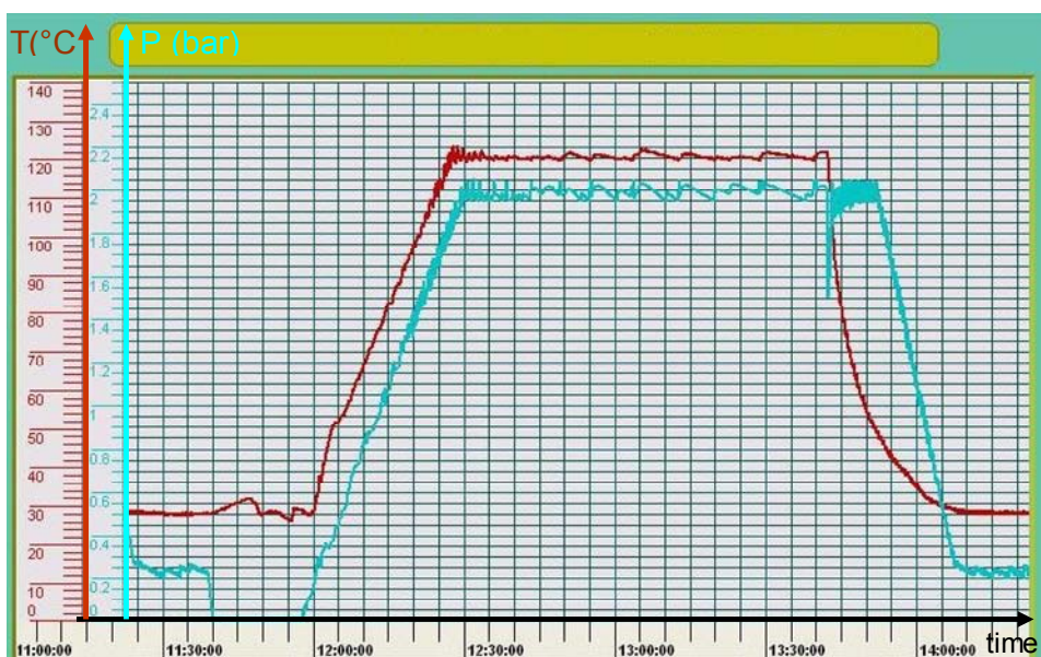
Figure 5: Picture file about a sterilizing process in an autoclave
