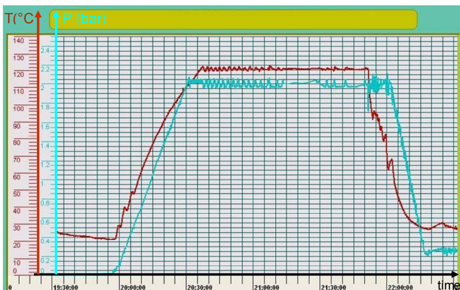
Figure 6: Insufficient steam supply
