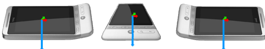
Figure 2: Equivalent orientations for the g-sensor
