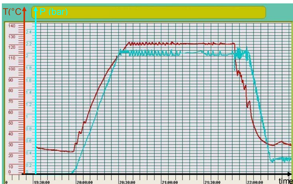
Figure 6: Insufficient steam supply
