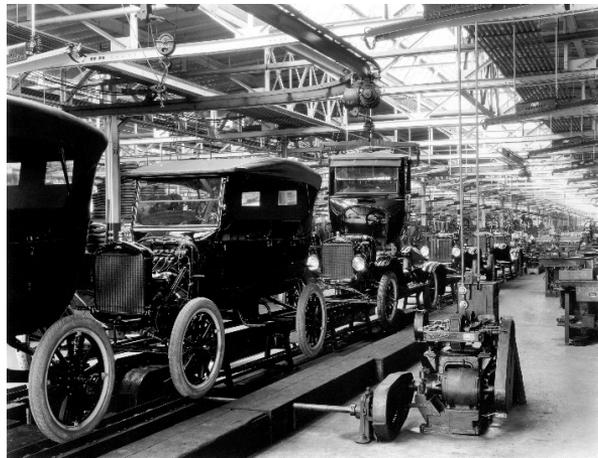
*Figure 2. Ford T-modell series production (source: supercompressor)*
