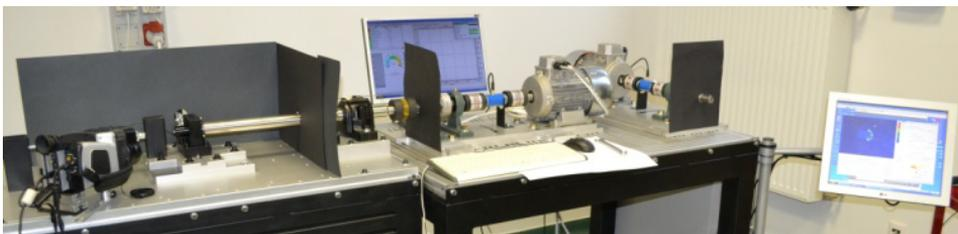
*Figure 2. Special purpose equipment for testing non-metallic bearings*
